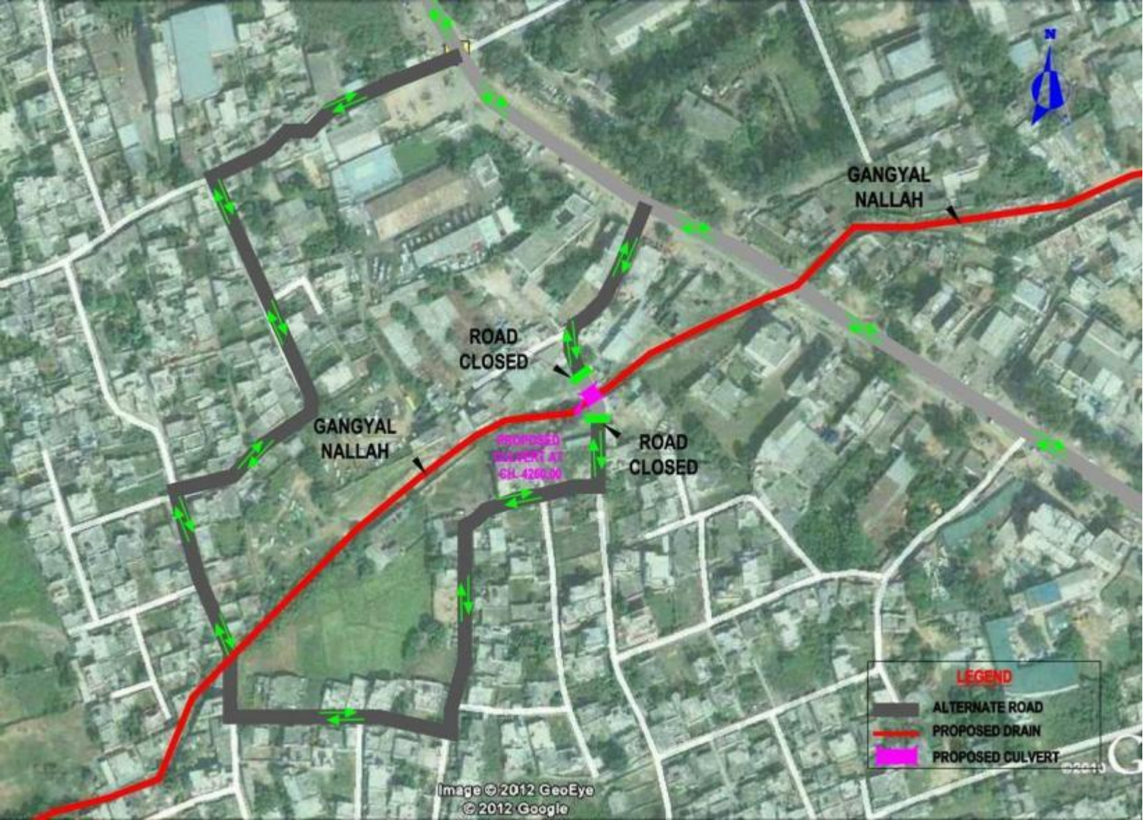
Diversion Map-B- Diversion Plan for Culvert site at Chainage-4260 m
