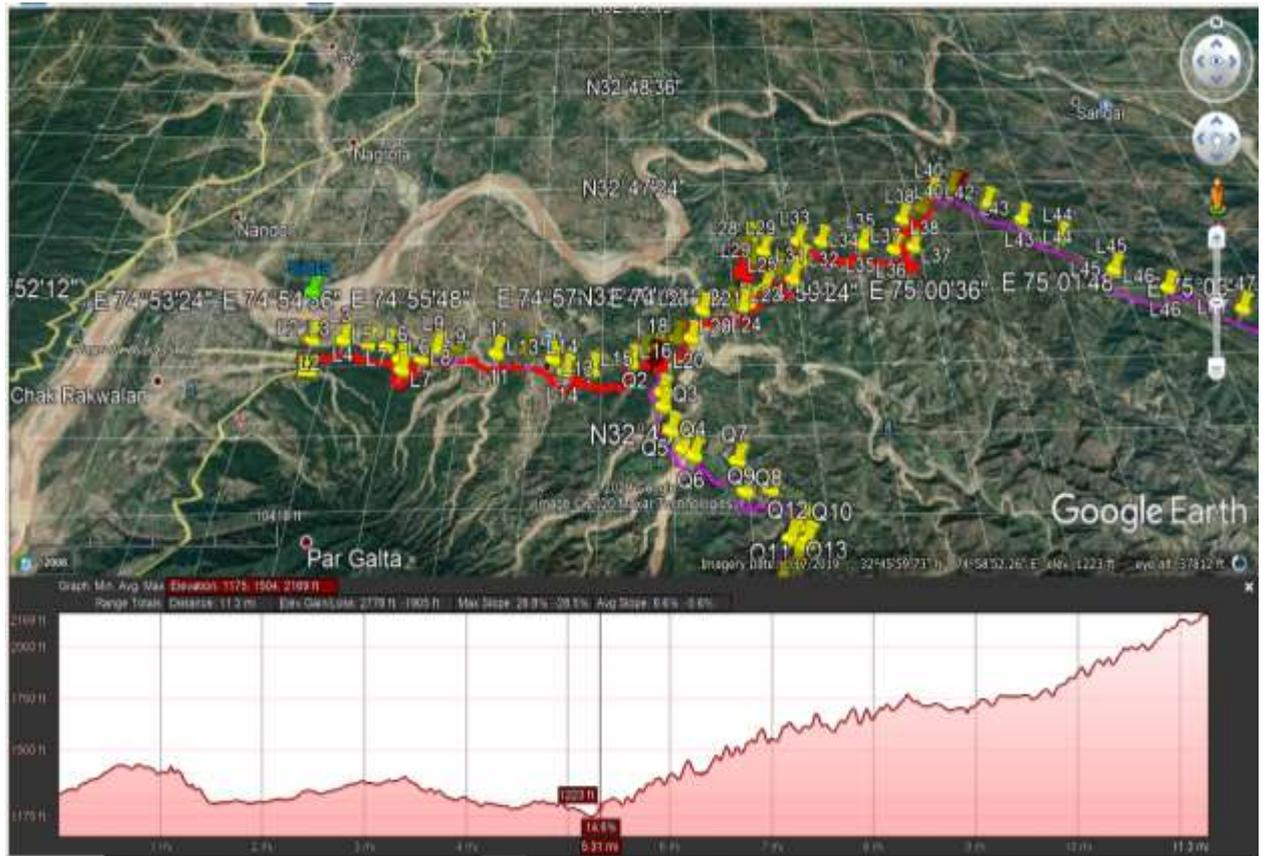
Fig 5.3: Elevation Profile of the proposed road from Sidra-Surinsar. (Source: Google Maps- Elevation details)
