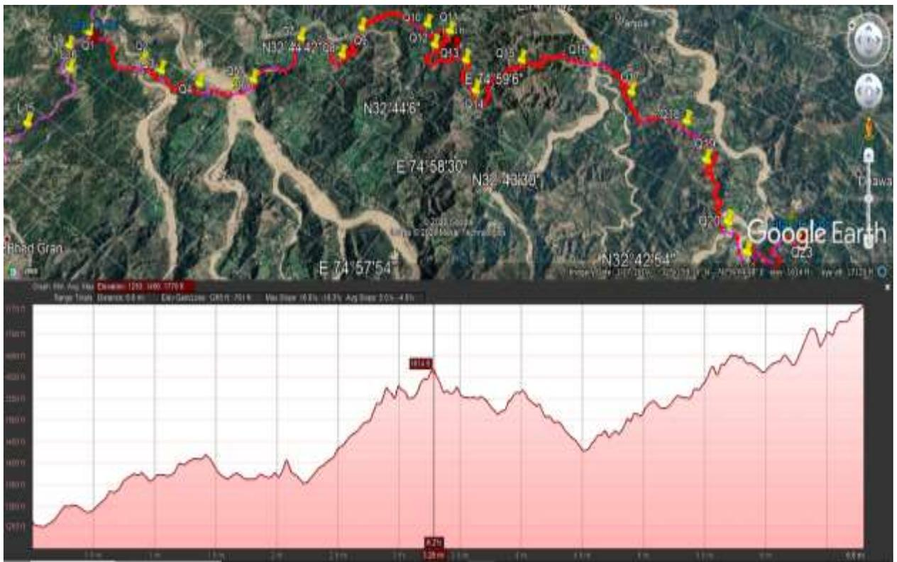
Fig 5.4: Elevation Profile of the proposed road from Tutan Di Khui. (Source: Google Maps- Elevation details)
