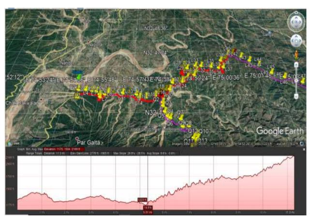
Fig 5.3: Elevation Profile of the proposed road from Sidra-Surinser. (Source: Google Maps-Elevation details)
