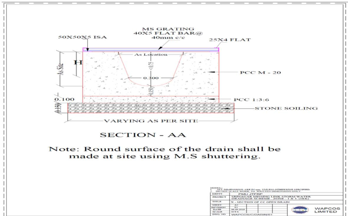
Fig 3.3: Cement Concrete Drainage Section
