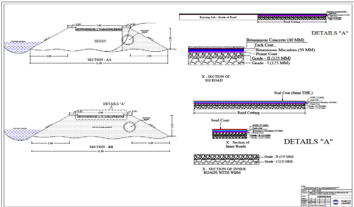
**Figure 3.6: X-Section of the Road Restoration Works**
