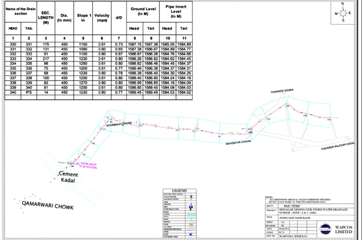
Fig 3.3: Index Map of the Proposed Storm Water Drainage Network in Noorbagh.
