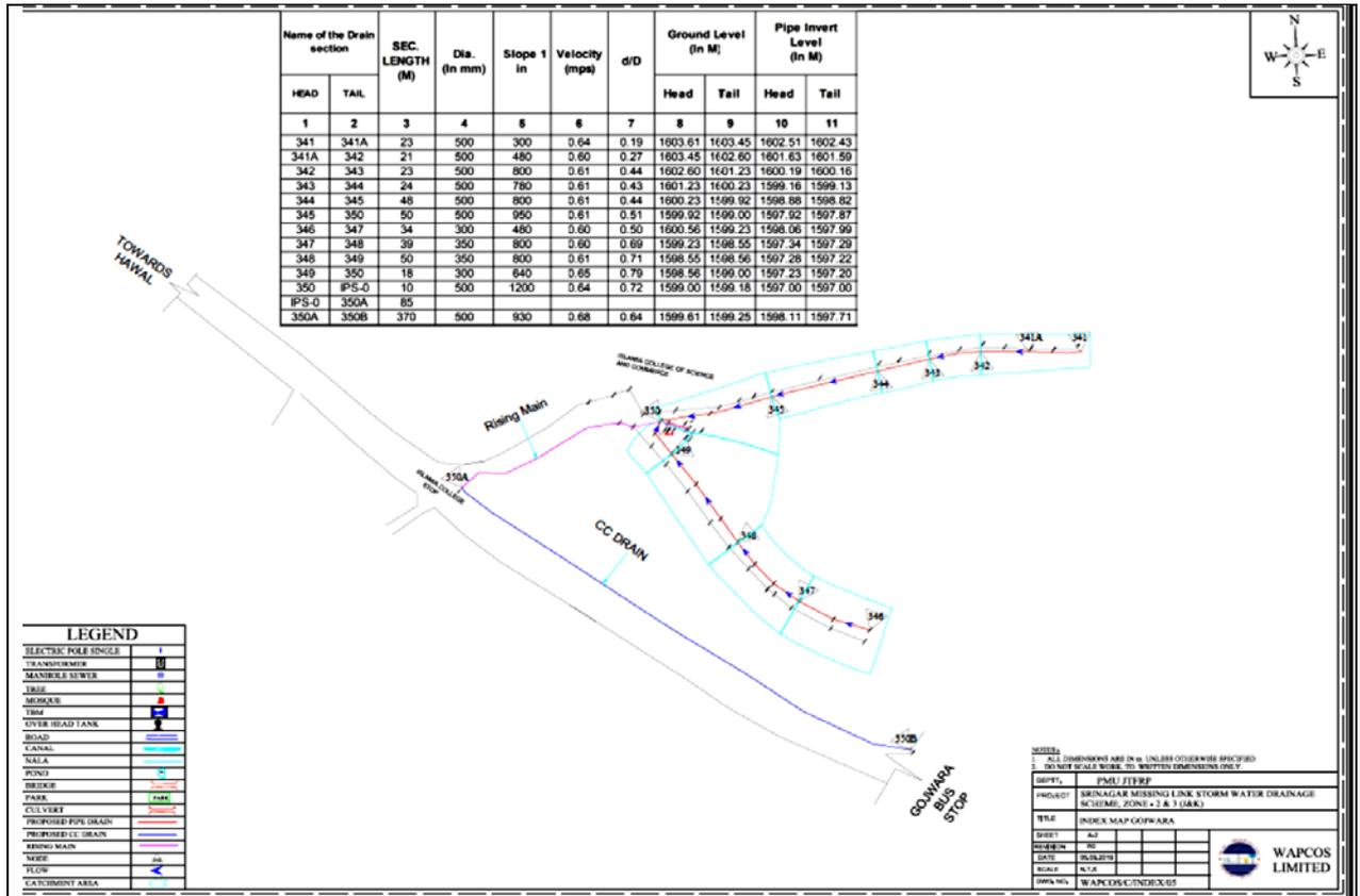
Fig 3.5: Index Map of the Proposed Storm Water Drainage Network in Gojwara.
