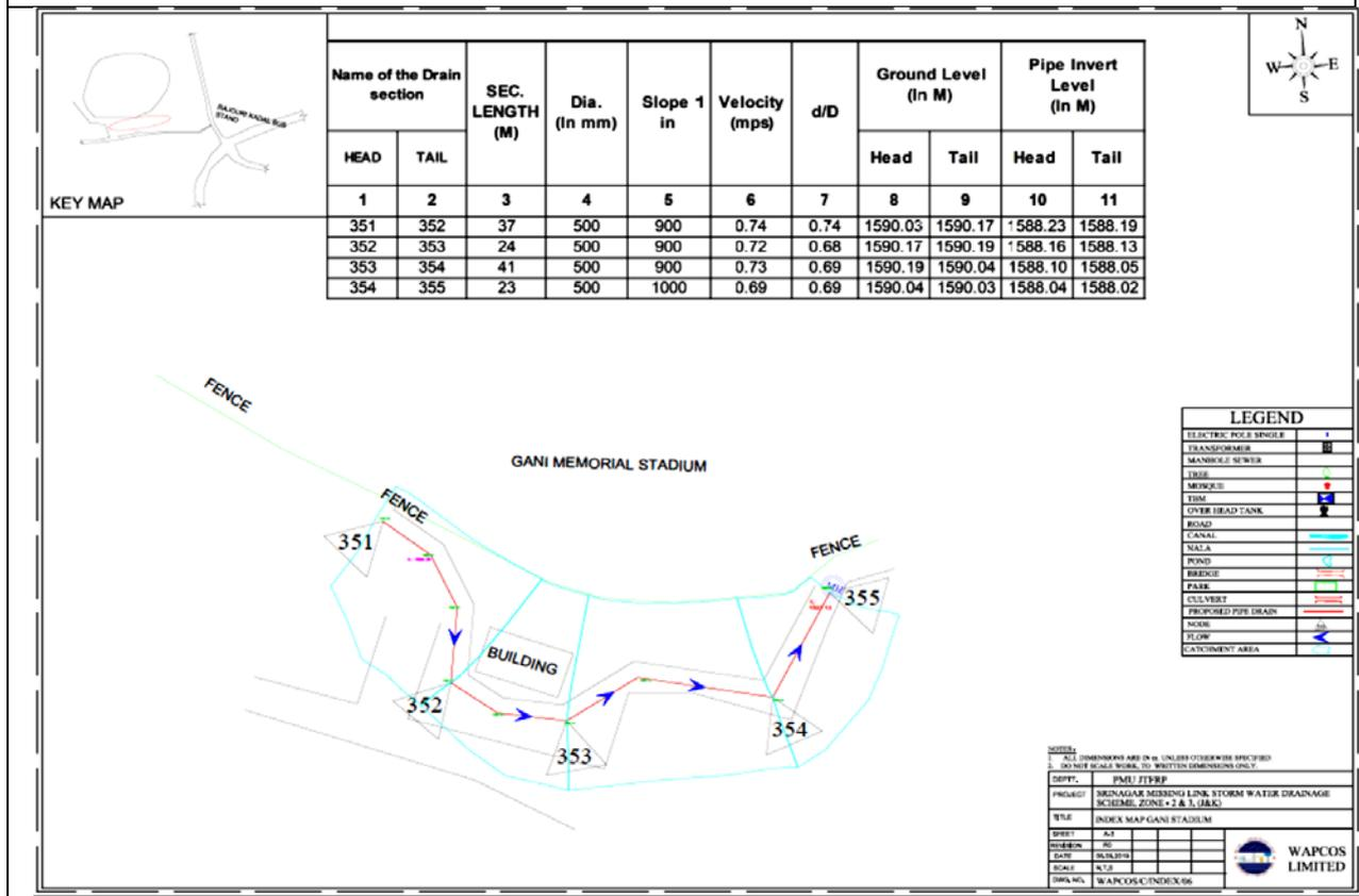
Fig 3.6: Index Map of the Proposed Storm Water Drainage Network at Gani Stadium side
